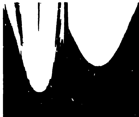
FIGURE 3. SMEAR CAMERA RECORD OF THE BREAKOUT OF THE TWO DIVERGING SPHERICAL WAVES GENERATED BY THE TEST ASSEMBLY SHOWN IN FIGURE 2. CLEAR PAINT WAS USED TO PROVIDE A SHARP TRACK (TIME INCREASE) UPWARD.
